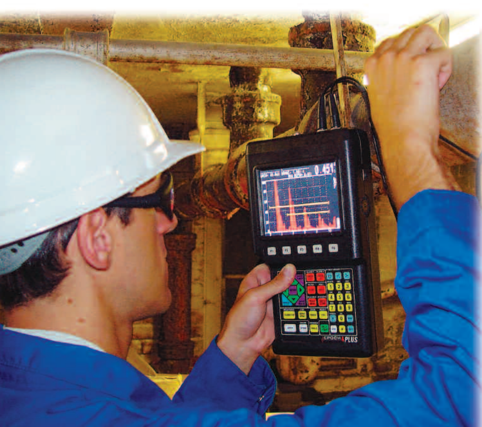
RF Echo-Echo thickness measurement with user-defined polarity detection
